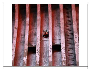
Thickness measurement carried out by a crawler
